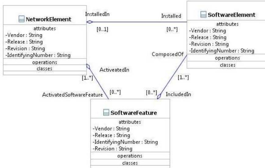
Figure 2. The meta-model of features, software and network elements defined using UML
