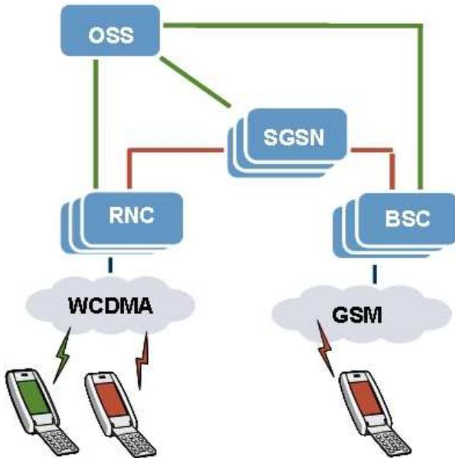
Figure 1. Nodes involved in SGSN In Pool feature.
