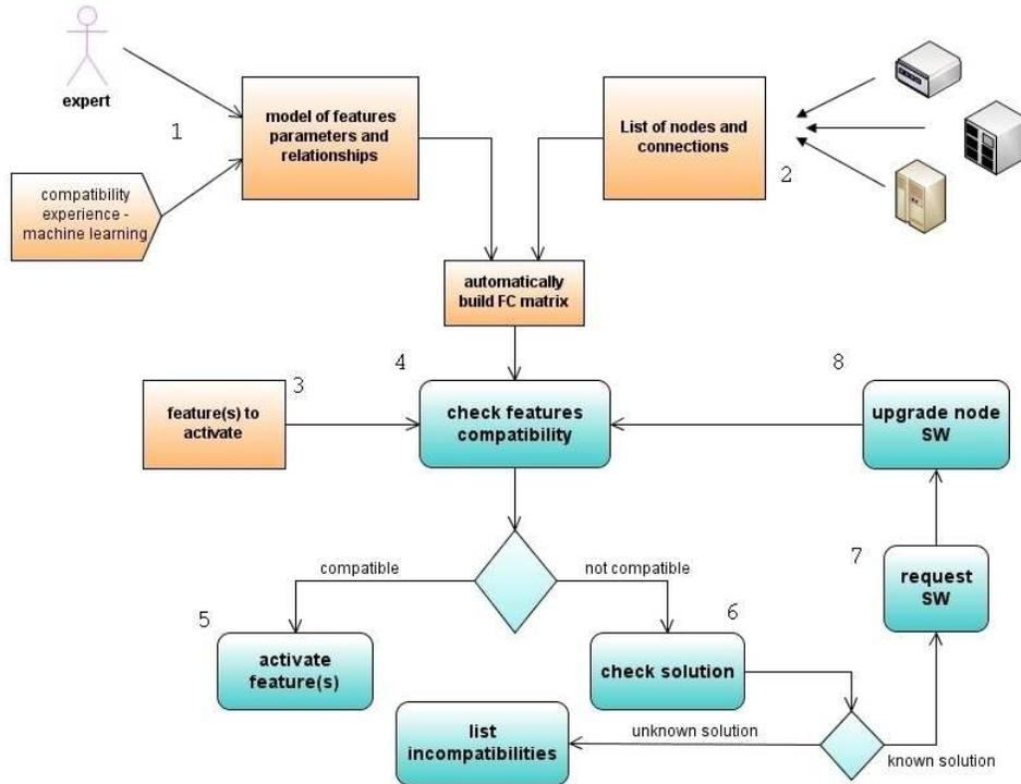
Figure 4. Proposed method of automatic feature compatibility assessment.
