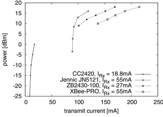
**Figure 1. Current consumption in transmission (for different RF power levels) and reception ( $I_{Rx}$ ) of existing WSN modules: CC2420 (voltage supply 3V), XBee-PRO (3.3V), Jennic JN5121-000-M02 (3V), ZB2430-100 (3.3V).**
